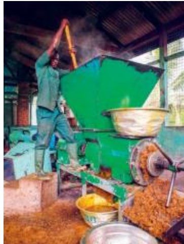
The oil press generates a by-product: a mixture of fibrous pulp and kernels to be processed further.
