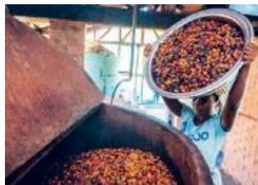
Oil palm fruits cannot simply be pressed, like olives, but have to be steamed for up to two hours first.
